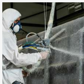
6. Fibreglass and resin spraying
