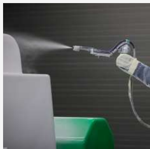
2. Application of the gelcoat, which will give the pool its colour
